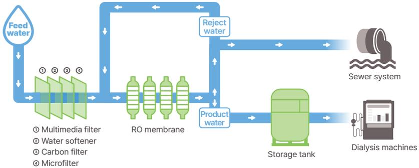
**Figure 1** Reject Water production during Reverse Osmosis and its subsequent disposal
