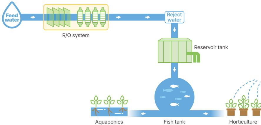
**Figure 3** Reuse of Reject Water in Malaysia
